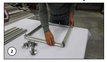
Make sure you have all the required material to assemble your light box. Position flat on a table the four extrusions to assemble the frame.
